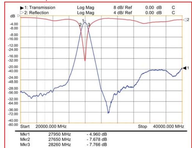
Above plot shows an example of our capabilities. This is a 3 poles SMT filter, centered at 27.95 GHz, BW 610 MHz (2.2 %), and return loss greater than 10 dB. Size (L x W x H): 1" x 0.250" x 0.030".
